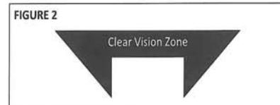
The clear vision zone is intended to provide for unobstructed visibility for vehicles and pedestrians. The clear vision zone is defined in accordance with the above illustrations and contains the area within the dashed lines. Figure 1 shows the dimensional calculations of the clear vision zone while Figure 2 shows the resulting shape of the clear vision zone.
